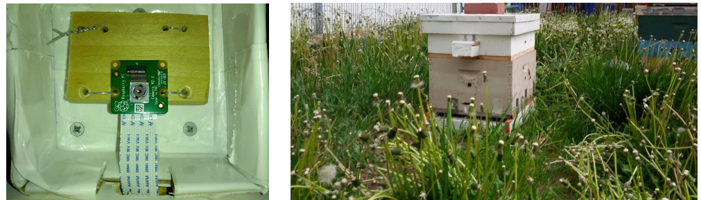
Figure 3. Left: A low-end, low-energy 8-megapixel Raspberry Pi camera v2.1 inside a waterproof camera protection box attached to the front of the super with the on-hive BeePi logger shown in the right picture. Right: An on-hive BeePi logger on top of a one super hive in Logan, Utah in May 2023; bottom to top: (1) a bottom board with a landing pad; (2) a light gray super; (3) a white super with the logger hardware shown in the left image of Figure 2, and a white waterproof camera protection box with the Pi camera in the left image; (4) a white telescoping hive lid.
