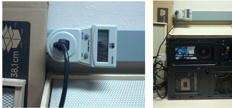
Figure 8. Left: A Gardner Bender(TM) PM3000 power meter plugged into a wall outlet. Right: A GEFORCE GTX-980 GPU computer plugged into a PM3000 power meter.
