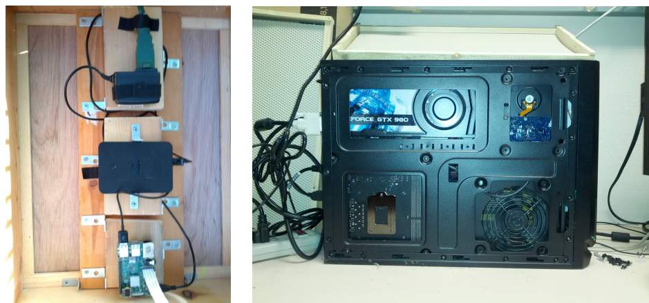
Figure 2. Left: BeePi logger hardware; bottom to top: a Raspberry Pi computer coupled to an 8-megapixel Pi camera (see left image in Figure 3); a five terabyte USB disk for archiving data for redundancy in case of GPU computer failures or power supply disruptions; a Pi power charger plugged into a waterproof power cord; videos are wirelessly transferred to a GPU computer over an ad hoc 802.11 local network, where they are processed and archived for redundancy in case of logger storage failures. Right: GEFORCE GTX-980 GPU computer (Arc: x86_64; CPU Family: 6; Model: 60; Model Name: Intel(R) Core(TM) i7-4790K; CPU at 4.00 GHz; BogoMips: 7999.890) with Ubuntu 18.04; all YOLO models were trained on this computer and evaluated for their energy efficacy and operational energy footprint.
