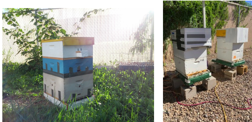
Figure 1. Left: An on-hive BeePi logger on top of a 2-super Langstroth hive in Logan, Utah; bottom to top: (1) a landing pad; (2) a light gray super; (3) a blue super; (4) a white super with the BeePi logger hardware (see the left image in Figure 2); (5) a waterproof plastic box with a Pi camera inside (see Figure 3) looking down on the landing pad; the box is attached to the front of the third super with two screwed metallic brackets; (6) a wooden migratory hive lid on top of the third white super. Right: two BeePi loggers on top of two super Langstroth hives in Tucson, Arizona; the top boxes on hives contain the logger hardware; water- and dustproof boxes on top of the second supers protect the cameras against rain and dust storms frequent in that area of Arizona.
